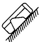
It is not possible to install at an angle of 40°~50° if only (A) is used. /
